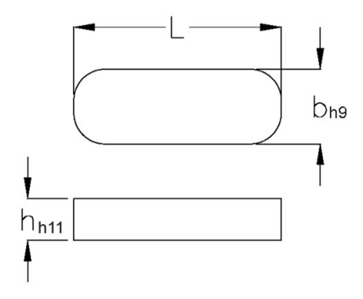
$\begin{array}{ll} b & = 8 \\ h & = 7 \\ L & = 63.0 \\ Tolerance \ b = 0.036 \\ Tolerance \ h = 0.090 \\ Tolerance \ L = -0,3 \end{array}$
